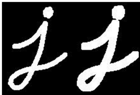
Fig.1.7. Before dilation[14] Fig.1.8. After dilation[14]
