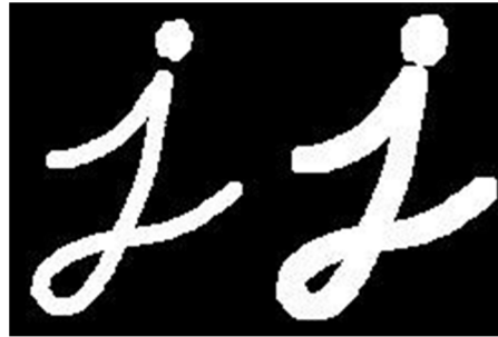
Fig.1.7. Before dilation[14] Fig.1.8. After dilation[14]
