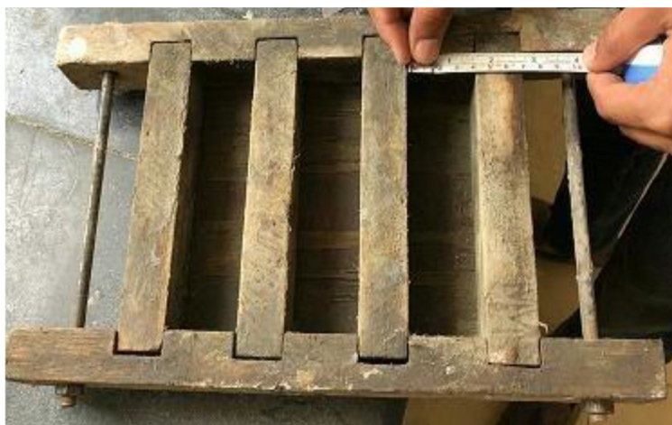
Fig 2. Moulds for Prisms of Size 40mm*40mm*160mm.
