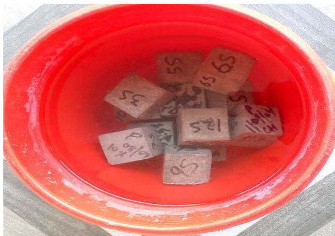
Fig 3: Immersion of Samples in 14% Solution of Sodium Sulphate Decahydrate
