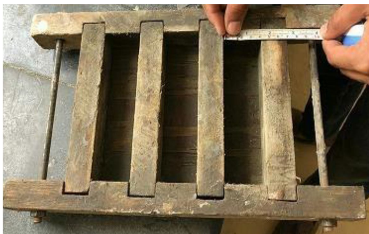
Fig 2. Moulds for Prisms of Size 40mm*40mm*160mm.
