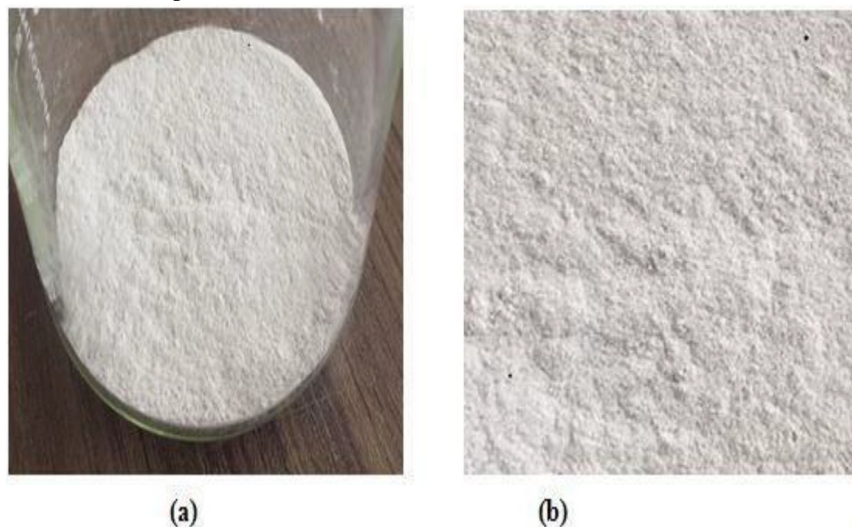
Fig 1: Wood Waste Ash Obtained from Open Burning.
