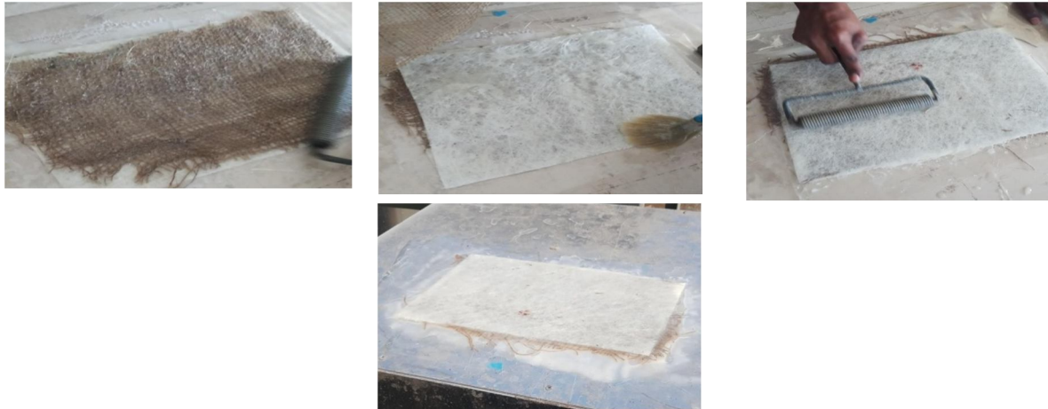
Figure 7. Fabrication by Hand-Lay Up Process
