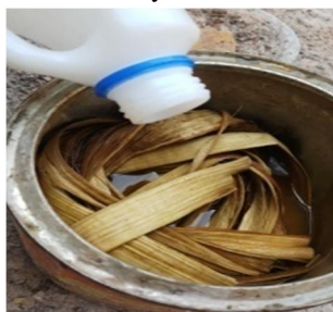
Figure 5. Surface Treatment of Fibers
