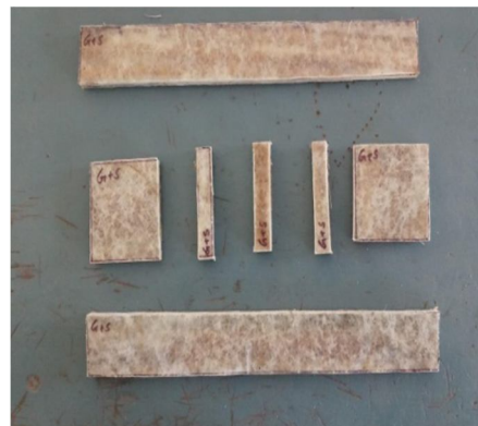
Figure 10. Glass Fiber + Screw Pine Fiber
