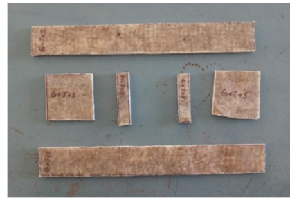
Figure 9. Glass Fiber + Jute Fiber + Screw Pine Fiber
