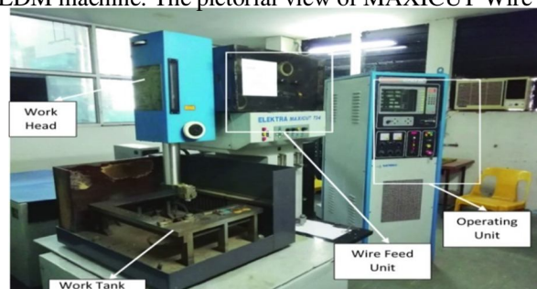
Figure 3.2 Pictorial image of Wire-EDM
