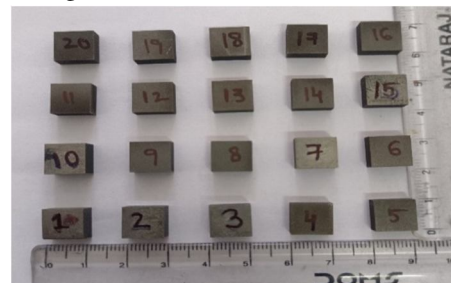
Figure 4.2 Machined samples using Brass wire
