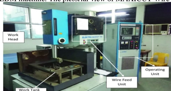
Figure 3.2 Pictorial image of Wire-EDM
