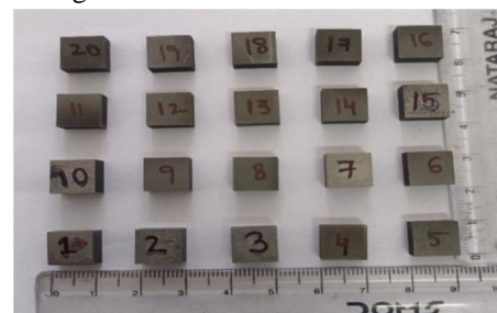
Figure 4.2 Machined samples using Brass wire
