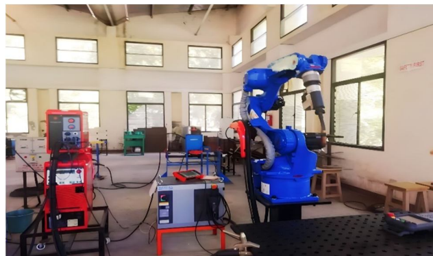
Figure 3.1 Pictorial image of WAAM
