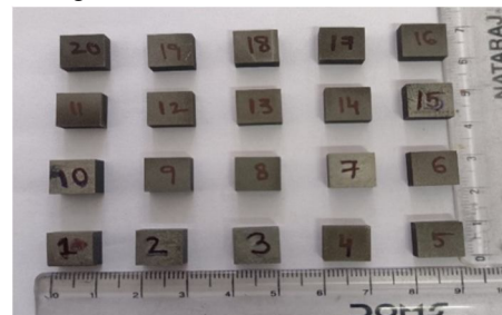
Figure 4.2 Machined samples using Brass wire
