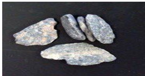
Figure :Flaky aggregates
