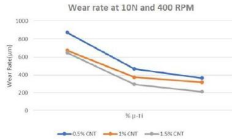
Figure 5.3 Wear rate of copper hybrid metal matrix composites, at 10N & 400 RPM
