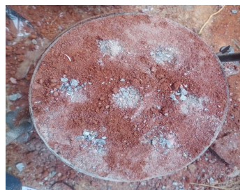
Figure.3: Soil with stone column arrangement
