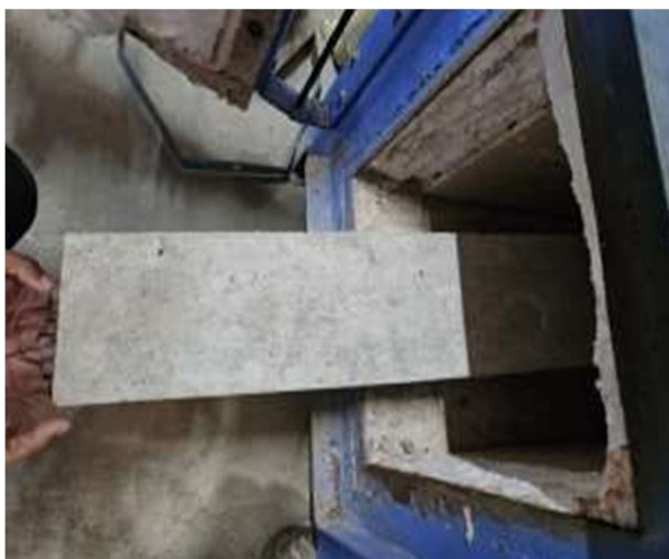
(a) Fired Process on Beam At (500°C)
