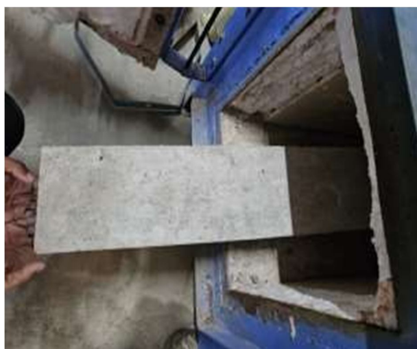
(a) Fired Process on Beam At (500°C)
