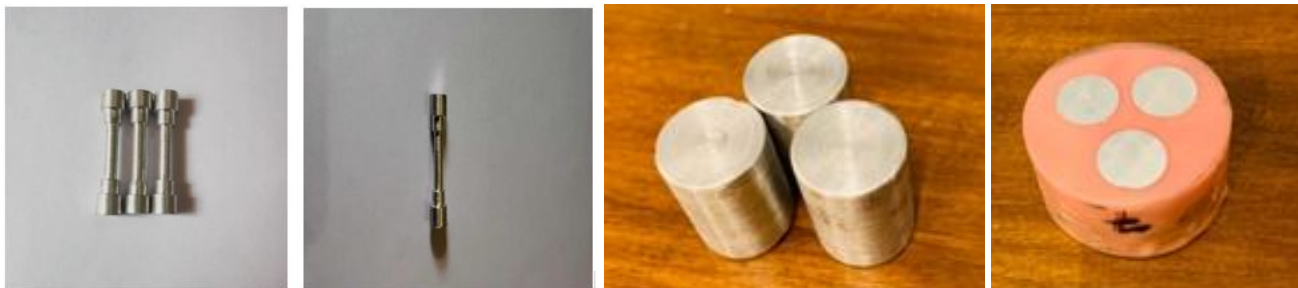
Figure 8: Specimen Preparation as per ASTM standard dimensions
