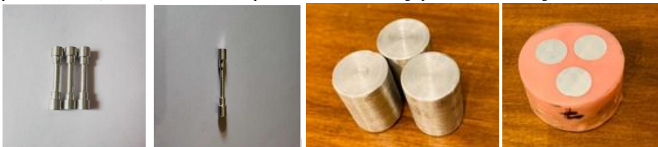
Figure 8: Specimen Preparation as per ASTM standard dimensions
