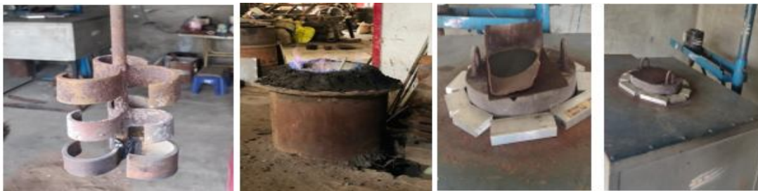
Figure 6: Stir casting Setup Used
