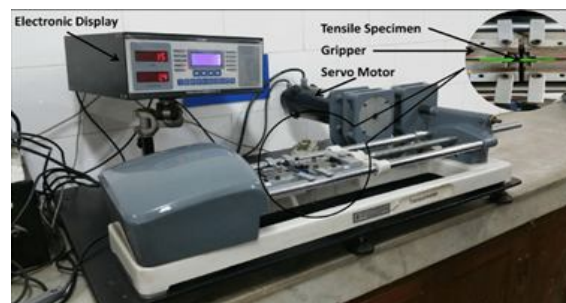
Figure 9: Tensile Testing Equipment
