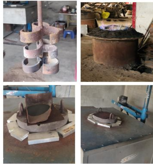
Figure 5: Stir casting Setup Used
