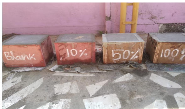
Fig: 3.2 Concrete cast at various proportion
