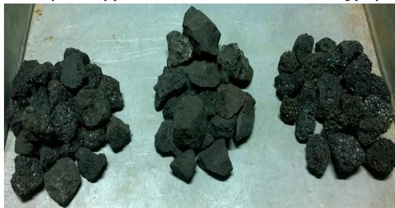
Mixed Slag Aggregate (SM) Heavy Slag Aggregate (SH) Light Slag Aggregate (SL)
