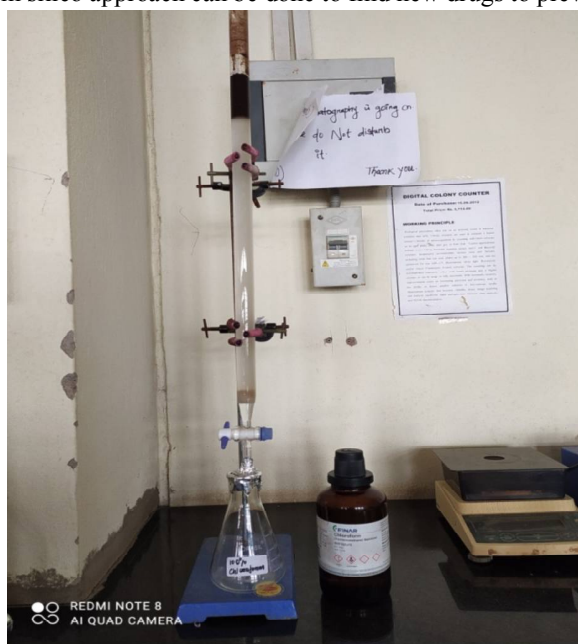
Figure 8: Column chromatography set up
