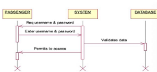
Figure 10. Sequence Diagram for Login
