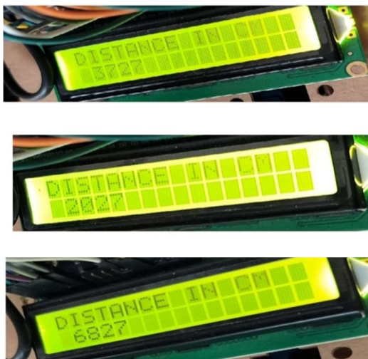
Fig 5: LCD display showing the distance of the obstacle measured by the robot
