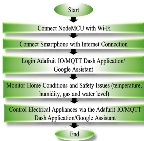
FIGURE 12. Flowchart of system operation.
