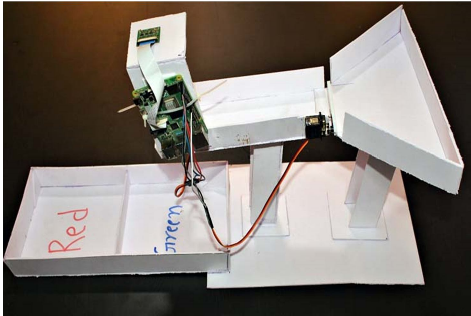
Fig8. Proposed Tomato Sorting Machine.
