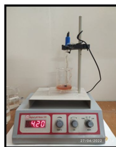
Fig.6 PH of tomato sample testing
