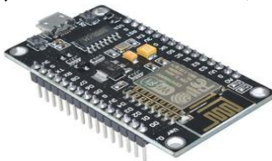
Figure 6: ESP8266 Wi-Fi module
