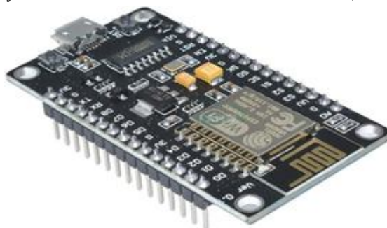
Figure 6: ESP8266 Wi-Fi module
