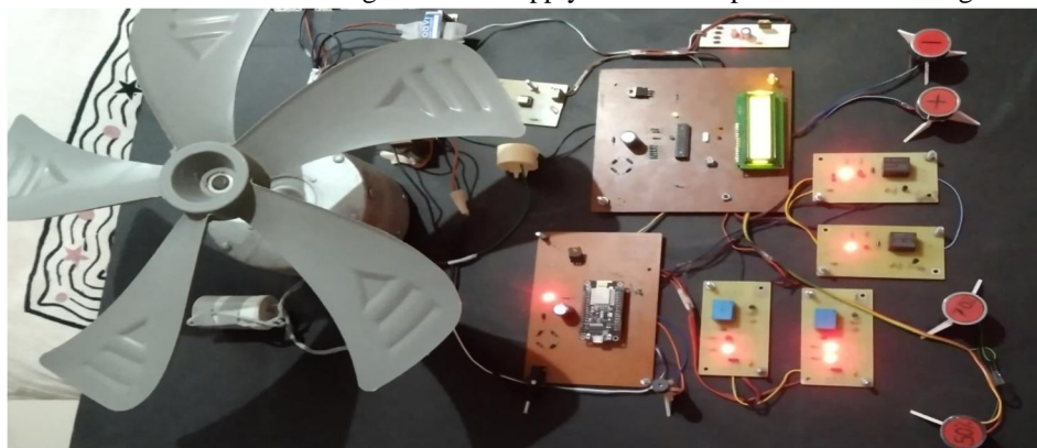
Fig. 10 Hardware set up of 1 phase induction motor model
