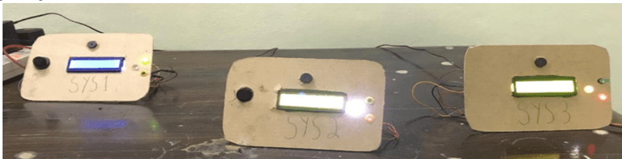
Figure 11.4 Overall setup during gas leak scenario
