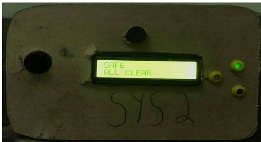
Figure 11. Gas detector 2 during clean air scenario
