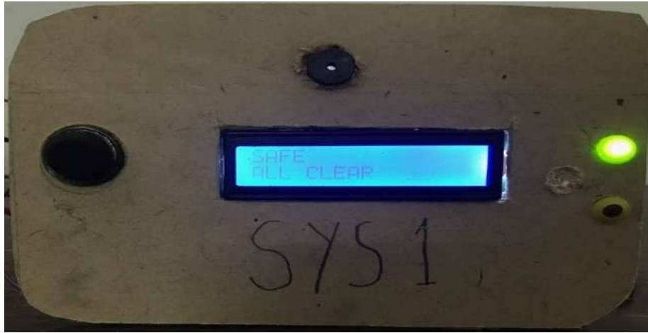
Figure 10. Gas detector 1 during clean air scenario
