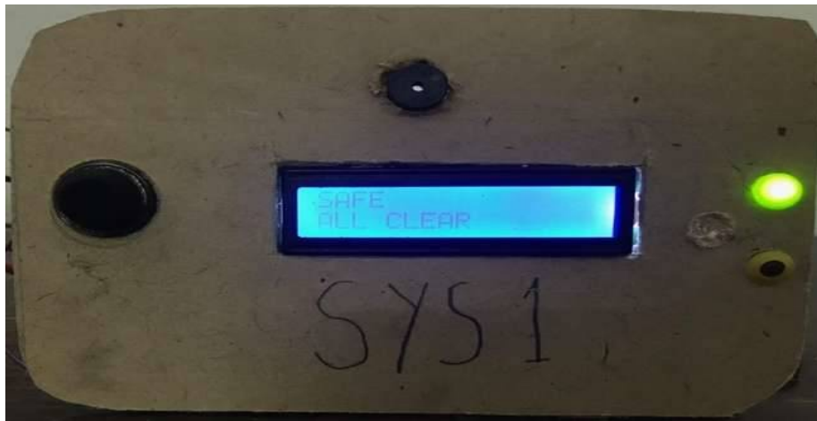
Figure 10. Gas detector 1 during clean air scenario
