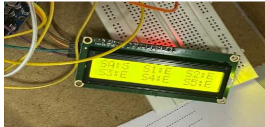
Fig 5: LCD Screen With Status Of Each Slot
