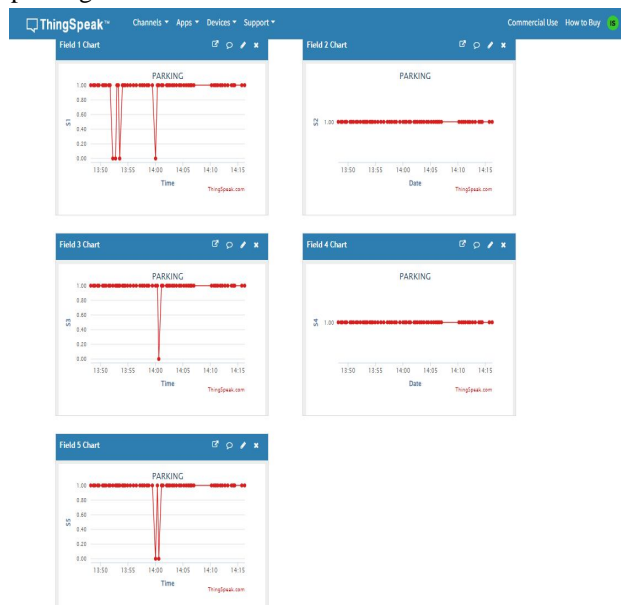
Fig 6: Dashboard of Thingspeak Showing Status Of Slots
