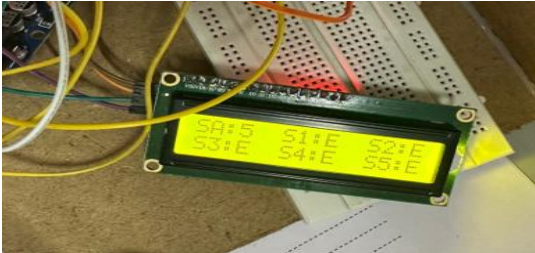
Fig 5: LCD Screen With Status Of Each Slot
