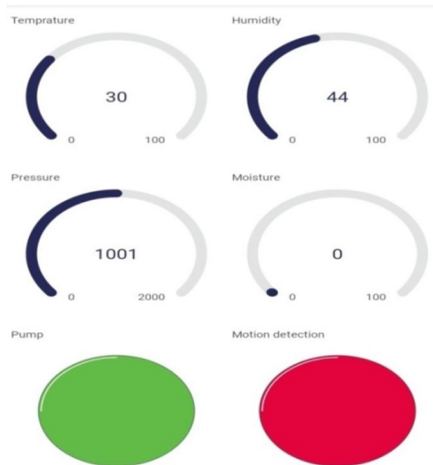
FIG. 8.6- Blynk App Output for Temperature, Pressure, Humidity and Pump State
