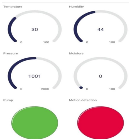
FIG. 8.6- Blynk App Output for Temperature, Pressure, Humidity and Pump State
