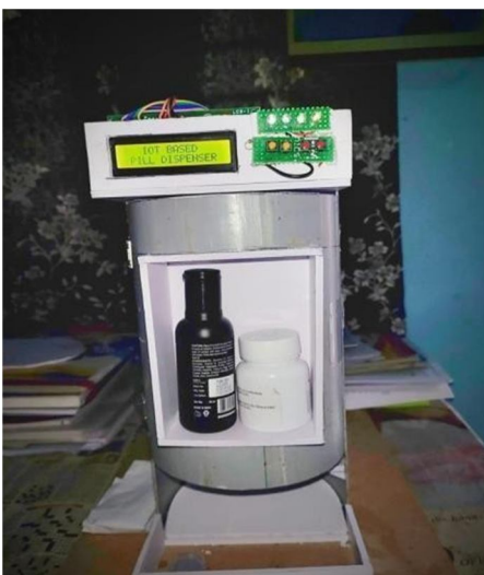
Fig.6 Front panel view of the medicine dispensing unit.
