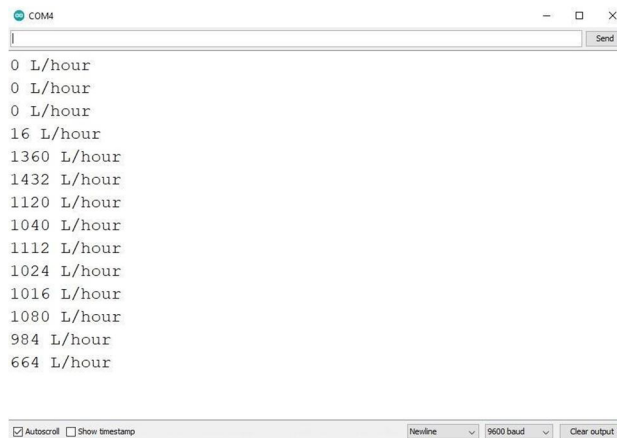
Fig. 3 Flow Rate Observation on Serial Monitor
