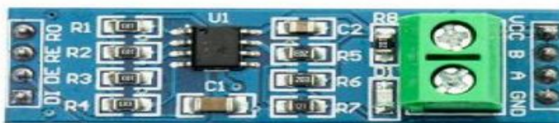
Fig. 2 Converter module for MAX485 TTL to RS485
