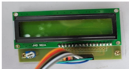
Figure 2. 16X2 LCD DISPLAY
