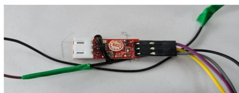
Figure 4. ARDUINO TURBIDITY SENSOR
