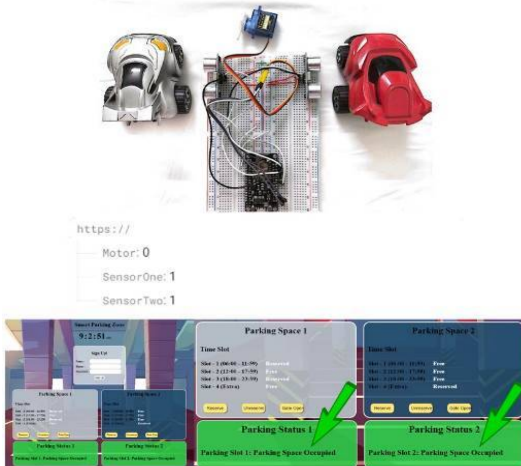
Figure 4.2. Live slot update status for occupied slots.
