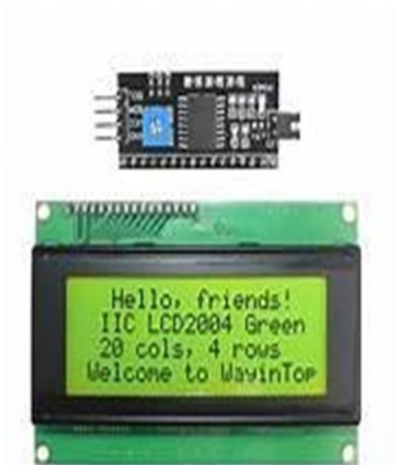
Figure 3.2.4 20X4 I2C LCD Display
