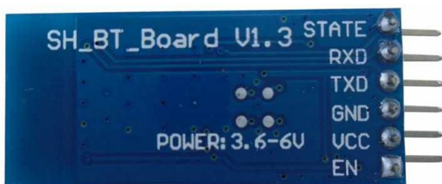
Fig 33.5.1.h.2 Pin Description of Bluetooth Module
