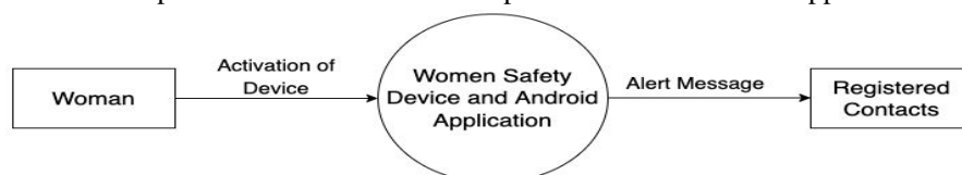
Fig. 2 Data Flow Diagram Level 0
