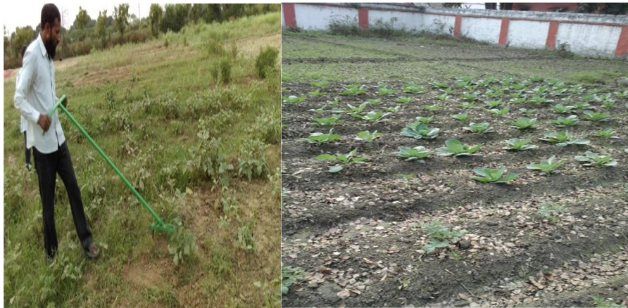
Figure 4.2 field evaluation of wheel hoe 2 and plant damage observed after 5 days of weeding.
