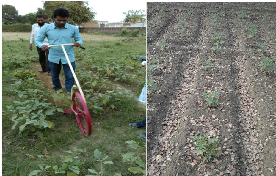
Figure 4.1 field evaluation of Three tyne wheel hoe and plant damage observed after 5 th day of weeding.
