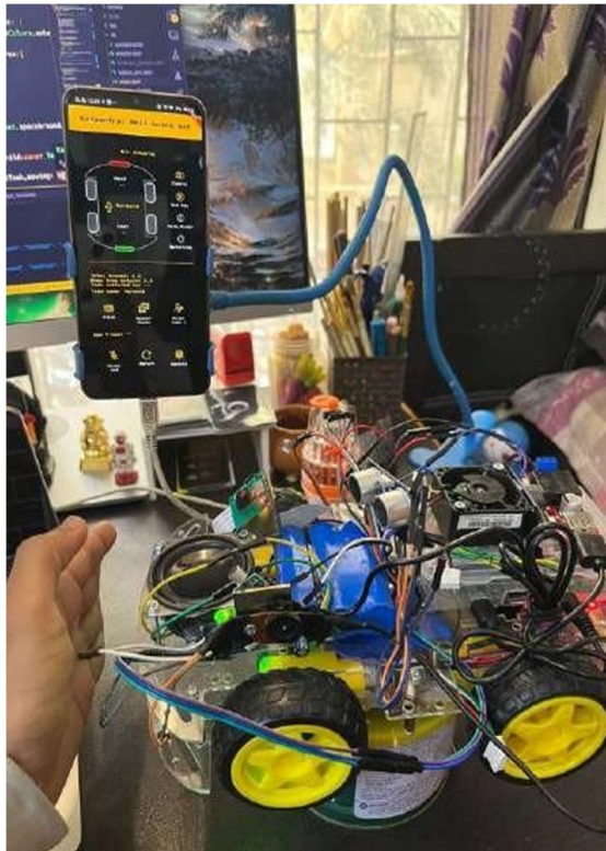
Fig.4 Kalyantra Example of Obstacle In Front and event sent to app Highlighted it.
