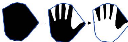
Figure 3. Convex hull Subtract the hand region to get regions between fingers
