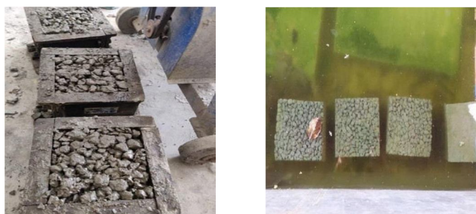
Figure 3.3 : Pervious Concrete Specimens and Curing of Pervious concrete
