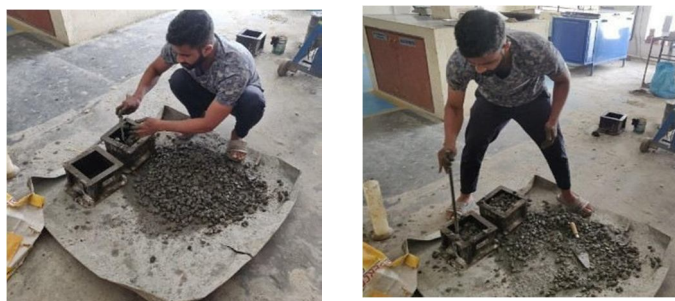
Figure 3.2 : Compaction of Pervious Concrete
