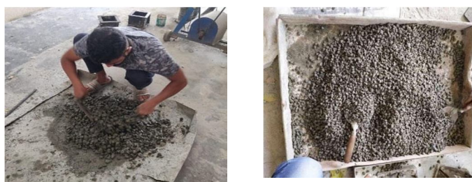
Figure 3.1 : Mixing of Pervious Concrete
