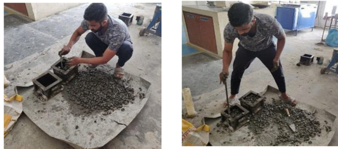
Figure 3.2 : Compaction of Pervious Concrete
