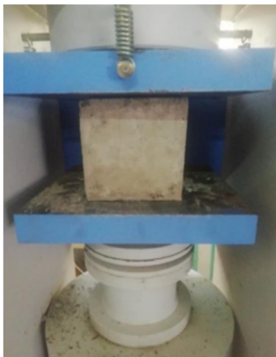
Figure-10: Compressive strength test
