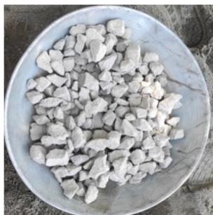
Figure-5: Recycled Aggregate From Lightweight Blocks
