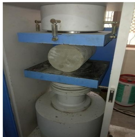
Figure-11: Testing of cylinder
