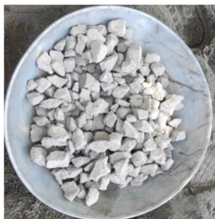
Figure-5: Recycled Aggregate From Lightweight Blocks
