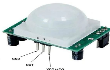
Fig 7 The above fig, shows a typical pin configuration of the PIR sensor.
