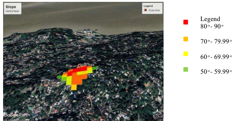
Fig. 2 Slope Mapping of Navagraha hill in GIS
