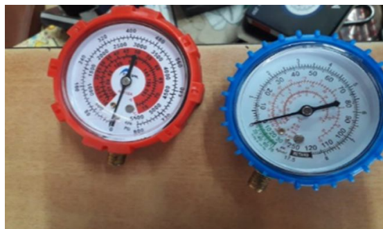
Fig. (c) Pressure & Vacuum Gauge
