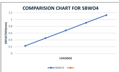
fig.5.c) Load vs Deflection curve for SBWO4
