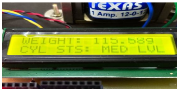
Fig6: when container is at medium level i.e., >60g and <200g
