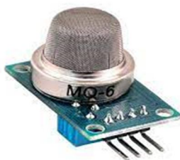
Fig 3: MQ-6 gas sensor
