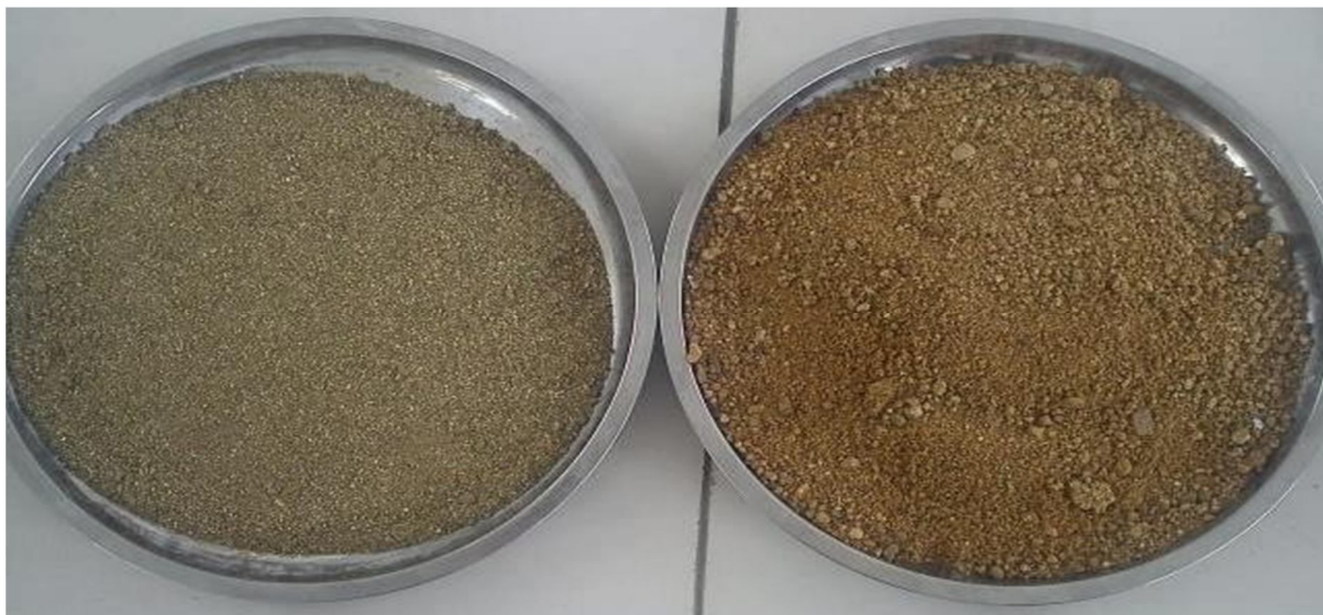
Iron Ore Slickens Natural Sand Figure 1: Comparison between natural sand and Iron Ore Slickens
