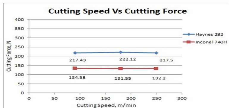
Fig. 9 Inconel 740H Vs Haynes 282; f = 0.05 mm/rev, \alpha = 8^\circ , r = 0.01 mm
