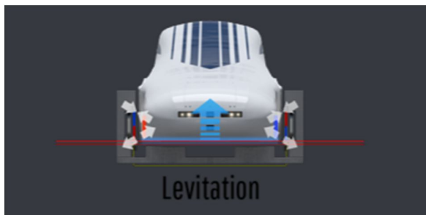
Fig.4 Principle of levitation, a mechanism to lift the train on the track.
