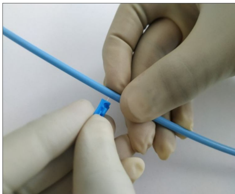
Figure.05 Manual punching process
