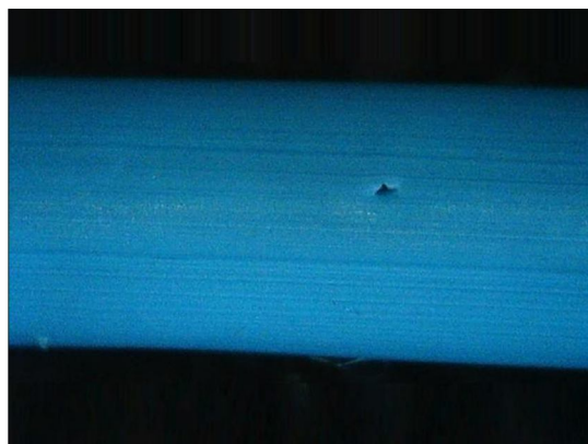
Figure.07 Microscopic Image of Hole on Infusion Catheter Perforated through Manual Punching Process
