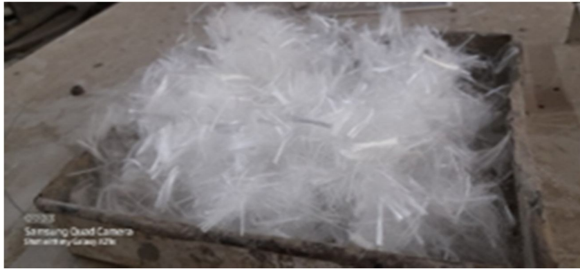
Fig. 3: 24mm monofilamental polypropylene fibre
