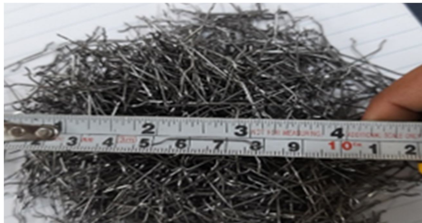
Fig. 2: End hooked steel fibre
