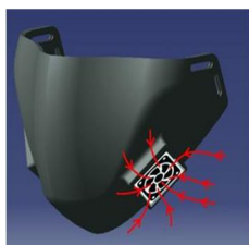
Intake Air Flow Through fan
