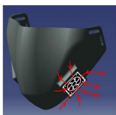
Intake Air Flow Through fan
