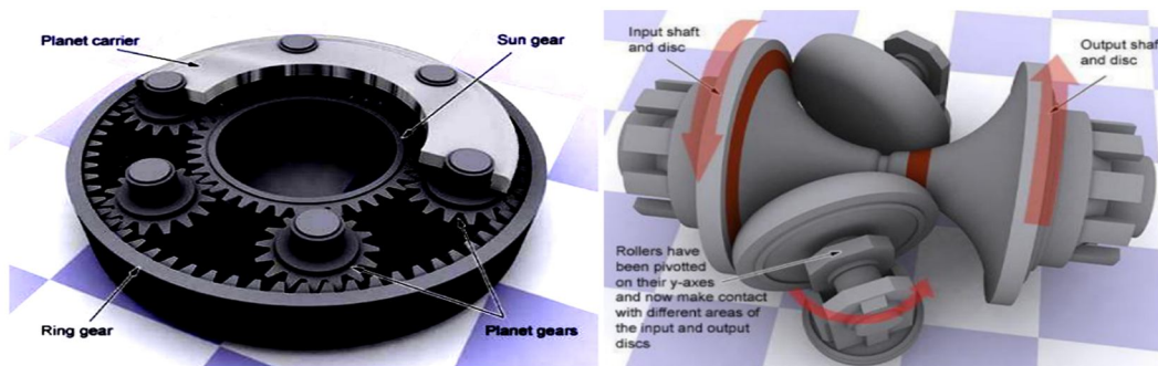
Figure -2: Planetary Gear System [6]
