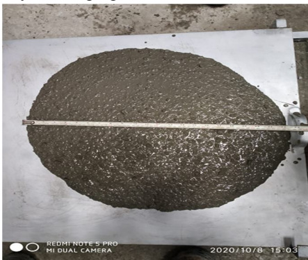
Fig.1 Slump Flow Test
