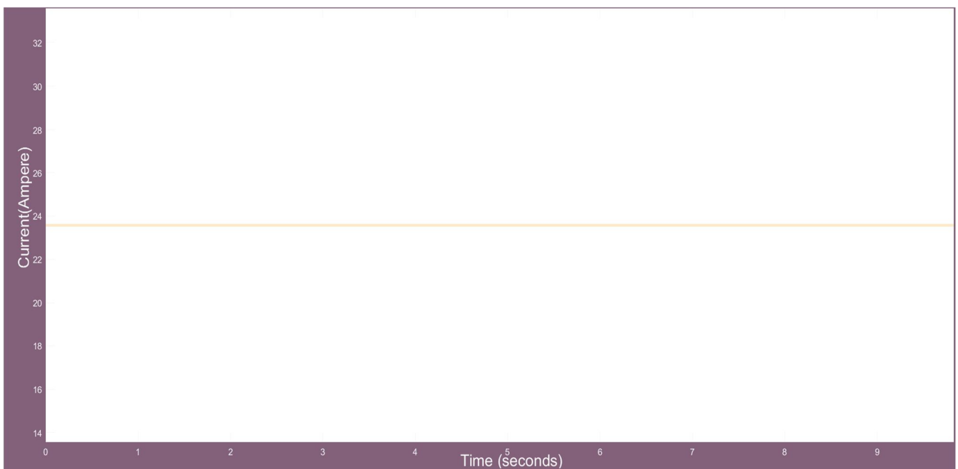
Fig 15 : Current curve of the PV modules under constant radiation
