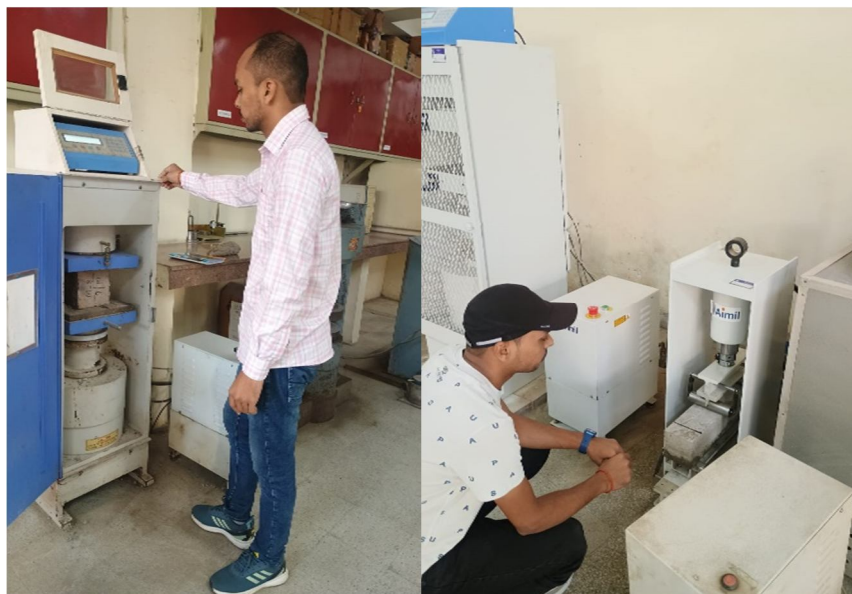
Fig.3 Compressive & Flexural strength test
