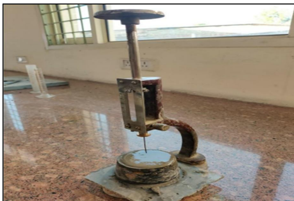
Fig.1 Initial setting time experiment on Vicat's Apparatus
