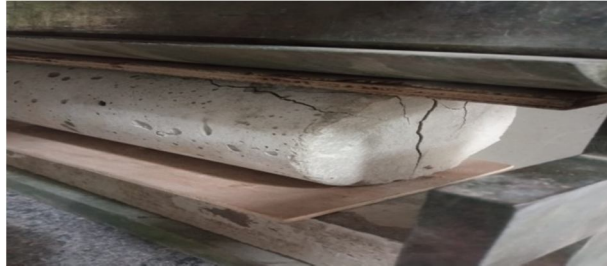
Fig.4 Split Tensile strength Test
